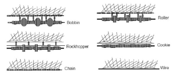
**Figure 4.2.**Examples of ground gear designs for bottom trawling. (Illustration from Buhl-Mortensen et al. 2013).
