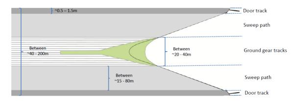
**Figure 5.1.** Conceptual footprint from standard otter trawls with three types of sea bed impacts: 1) the track affected by the otter boards (Door track), 2) the track influenced by the sweeps (Sweep tracks) and 3) the track affected by the trawl/groundgear itself (Ground gear tracks) (Illustration Buhl-Mortensen et al. 2013).
