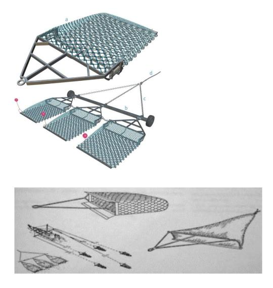
**Figure 4.7.** Different dredge types, with and without with shearing edge and teeth, and towed in different ways and numbers (drawings from O'Neill 2013 (top) and FAO Fisheries Technical Paper No. 419(bottom))
