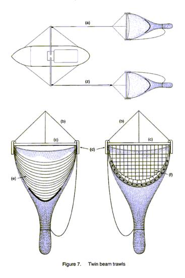
Figure 4.6. Top: towing two beam trawls: Bottom: bema trawls with different design of ground gear.
