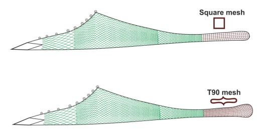
Figure 7.5.3. Different types of mesh in the bottom trawl codend
