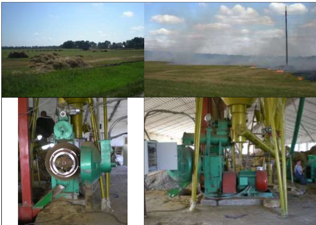
Figure 14. Tuzetka first focused on pelletisation of straw and export to Poland as illustrated in the pictures here showing how straw is currently often burned in the field and how it is pelletized in a small scale local pelletization plant.
