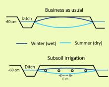
The increase in water level during summer from about -100 cm to -70 cm, was expected to reduce  $CO_2$  emission. An experiment in the Netherlands showed that the yield can improve slightly due to improved drainage during wet periods, so that the land is manageable earlier in spring. Reductions in  $CO_2$  emissions, however, were not found. The costs for this technique are  $\notin$ 9000,- per hectare (installation + maintenance).
