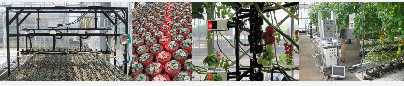
The Precision Spraying System (PSS) is a spray boom that moves through the greenhouse on a transport platform and sprays only there where needed. The PSS sprays only those areas in the crop where a sensor detected a diseased plant. The applied spray is adapted to the size and the density of the crop canopy.
