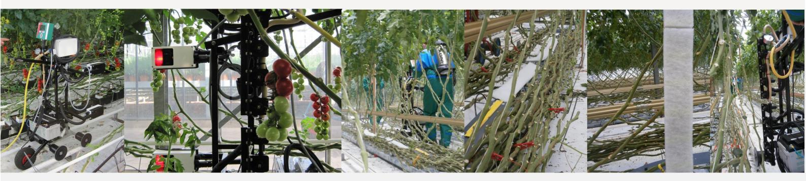
The Crop Adapted Spraying (CAS) sprayer sprays only there where it is necessary. The CAS-sprayer uses a sensor to detect the tomato stem and will spray it when a disease is to be controlled.
